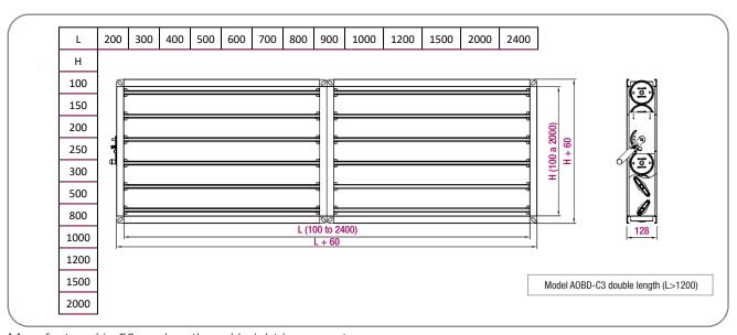
Manufactured in 50mm length and height increments.
