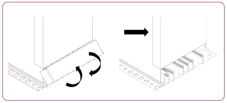
4.1B.2- Follow the instructions in part 3 above to install the plenum boxes in the positions required for each installation.
