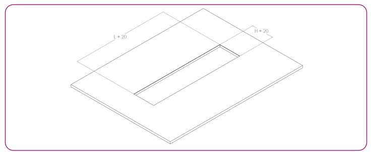
2.1- Cut an opening in the plasterboard (L+20) x (H+20)
