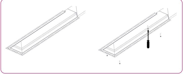
Where the plenum boxes are fitted independently of the grille, it is not necessary to fix them together. The plenum box should be fixed to the ceiling slab and the grille to the plasterboard. This allows supply and return air rows to be designed according to requirements of the project.
