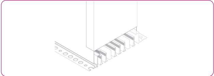
4.1A.2- Install the plenum box + grille assembly according to the instructions in part 3 above. Make sure the plenum boxes at the start/end of the row are installed first, followed by the intermediate plenum boxes.
